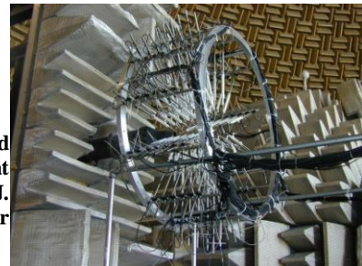
Figure 18 78 microphone near-field array, constructed and tested at NASA Glenn Research center by J. Bridges and S.-S. Lee. See [5] for further details.
